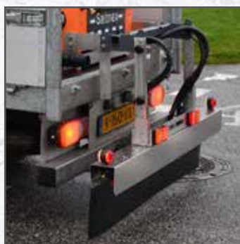
Stainless steel boom and nozzles
