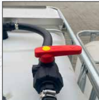
Three-way valve with two settings
