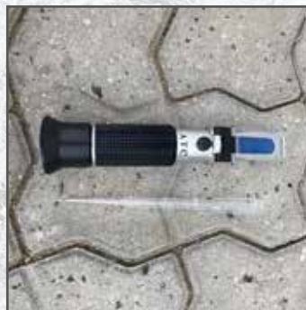
Refractometer and pipette for checking mixing ratio
